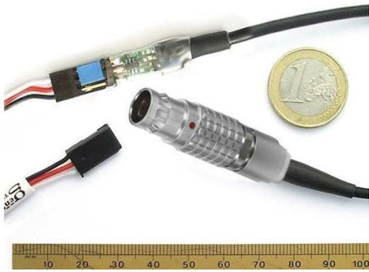
gentWIRE-ARRI allows control of record START/STOP on ARRI movie cameras.
