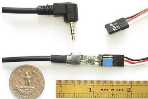
The gentWIRE-FOCUS. Allows control of focus AND shutter on cameras with electrical contacts.
