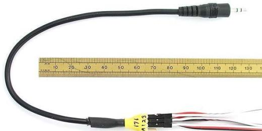
This device interfaces a Camcorder with a 2.5mm jack LANC interface (Sony, Black-magic, and some Canon models) with a RC receiver. Up to 2 RC channels can be used, controlling REC, PHOTO & **progressive ZOOM**.
