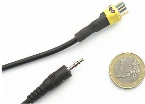
This device controls a Camcorder with a LANC interface via a RC receiver. Typically it is compatible with Sony and Blackmagic models. Up to 4 RC channels can be used, controlling REC, PHOTO, FOCUS, IRIS & ZOOM. Any number or combination of channels can be used.
