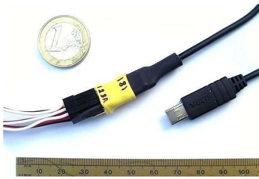
This device interfaces a Sony Camera with a MULTI interface with a RC receiver. Up to 3 RC channels can be used, controlling SHUTTER, REC, ZOOM, & ON/OFF.
