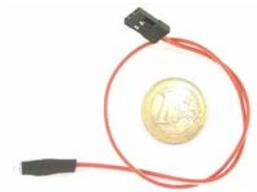
gentWIRE-multiAUDIO provides an audio indication of Camcorder status designed to be relayed via an audio channel of a video downlink. Tones tell the operator about REC, Memory, & Battery state.
