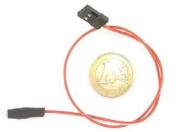
This device gives visual indication of camera status when connected to the AUX socket of gentWIRE-MULTI. Typically the LED gives the camera operator pre-flight and in-flight feedback on camera status.
