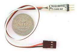
This device generates audio tones confirming Camera status when connected to the AUX socket of gentWIRE-MULTI.
