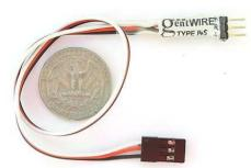
This device generates audio tones confirming Camera status when connected to the AUX socket of gentWIRE-redPRO. Typically this audio can be relayed to the camera operator on the unused audio channel of the video downlink.
