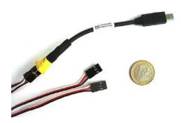
This device interfaces a Sony Camcorder with a AV or MULTI LANC interface with a RC receiver. Up to 2 RC channels can be used, controlling REC, PHOTO & progressive ZOOM. There is also access to the cameras video o/p.
