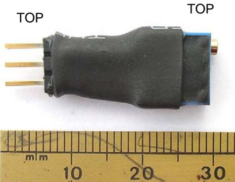
**genTIMER** is an intervalometer or timer for stills cameras. It is ideal for simple remote operation and triggers the camera between 2 & 30 seconds.
