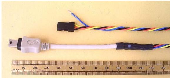
This device allows Canon cameras with the SDM / CHDK enhancement to be remotely triggered by a RC receiver. If your camera doesn't already have this enhancement then more information and scripts are
