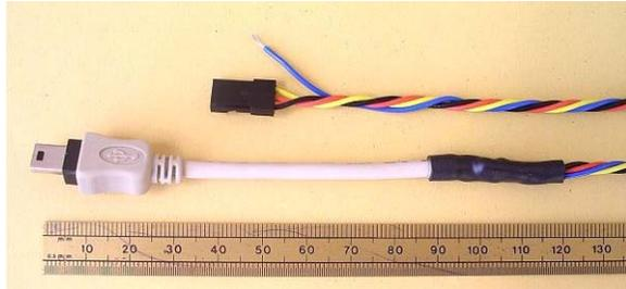
This device allows Canon cameras with the SDM / CHDK enhancement to be remotely triggered by a RC receiver. Up to 2 RC channels can be used, resulting in 7 different triggers to the camera.
